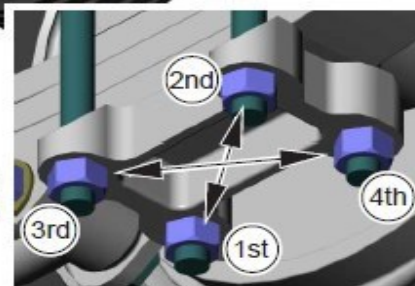
Item #5- Torque the axle u-bolts in the pattern shown.
